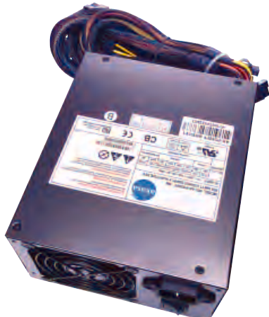
The power supply unit and its fan are crucial components for case cooling
